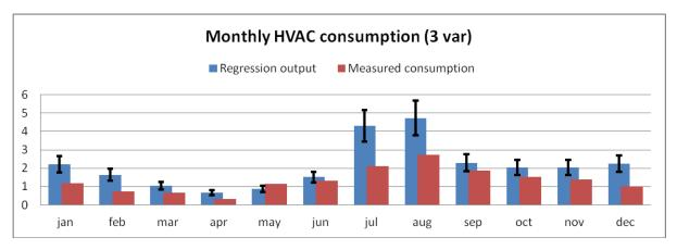
Figure 6: 3 variables model results (kWh/m<sup>2</sup>)
