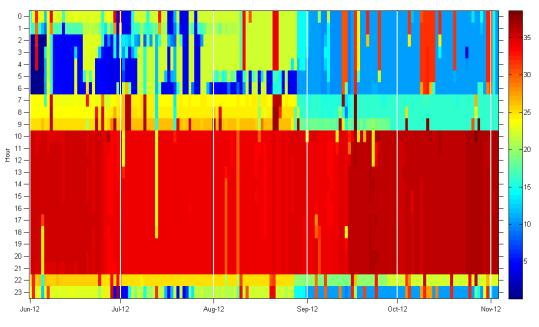
Figure 3: Lighting electric consumption of building G (kWh)
