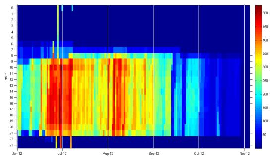
Figure 2: Rooftop electric consumption of building A (kWh)
