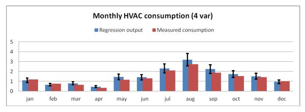
Figure 7: 4 variables model results (kWh/m2)
