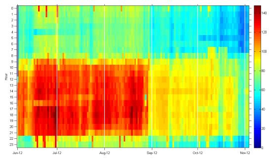
Figure 5: Food refrigeration (positive temperature) chiller consumption in building F (kWh)
